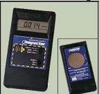
**Gamma Sensitivity:** 3500 CPM/mR/hr referenced to Cs-137. Smallest detectable level for I-125 is .02  $\mu$ Ci at contact.
